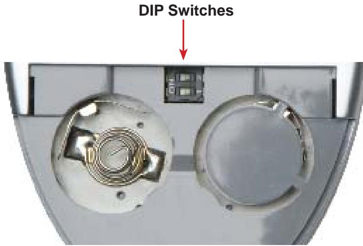
It is important that the IR channel selected on the remote, match the IR channel on the GefenToolBox 4x4 Matrix for HDMI 1.3 for proper operation. For example, if you set both DIP switches on the remote to the down position (toward the “1” and “2”), IR channel 0, you must set the GefenToolBox 4x4 Matrix with FST to use IR channel 0.
