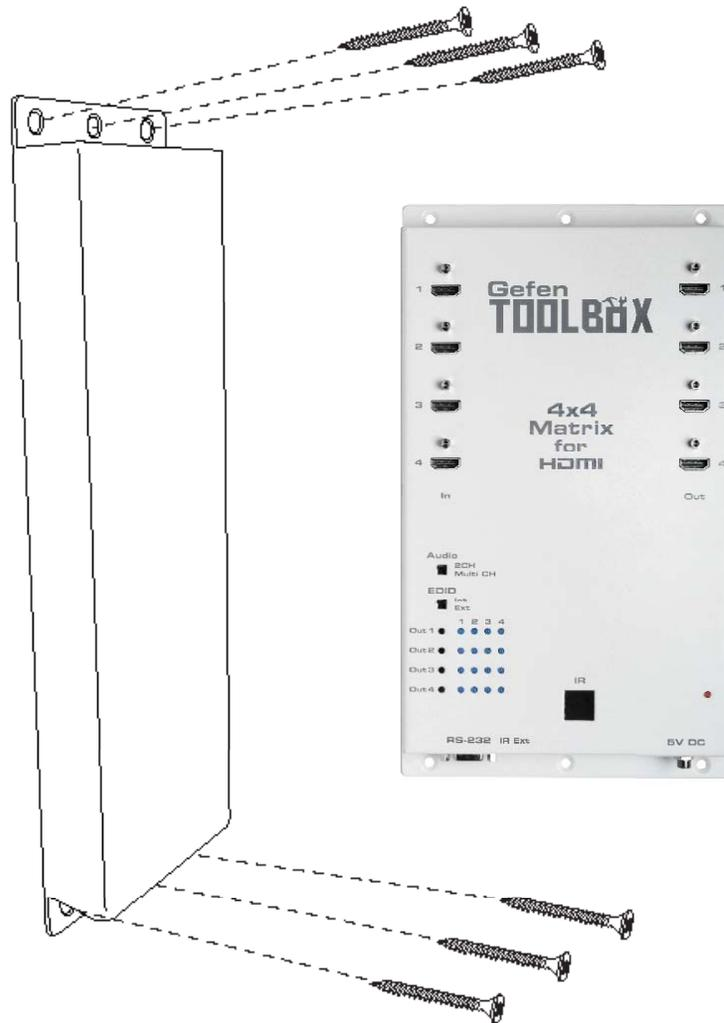
The GefenToolBox 4x4 Matrix for HDMI 1.3 should be mounted vertically in a wall or cabinet with wood/drywall screws as shown in the diagram above. There should be an inch or two of clearance between the edges of the unit and any walls or vertical surfaces to allow for enough clearance for insertion and retraction of cables at the HDMI connectors.
