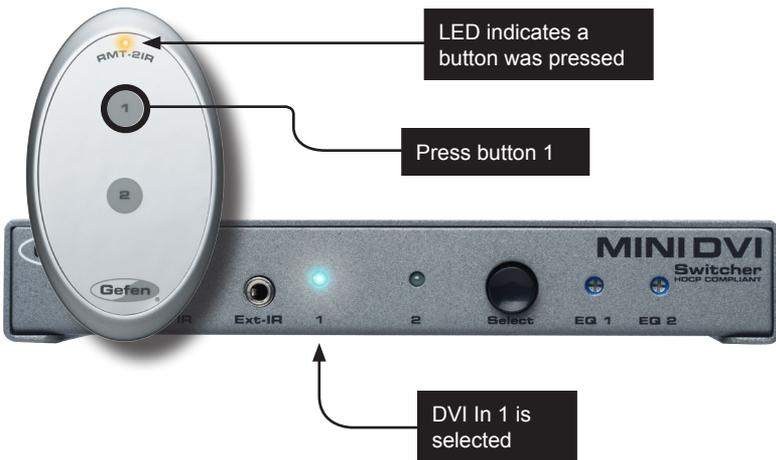
3. Pressing button 2 on the IR remote control unit will select **DVI In 2**. LED 2 will glow bright blue, indicating that **DVI In 2** is the active input.
