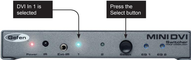
4. Pressing the **Select** button, again, will toggle the input to **DVI In 2**. LED 2 will glow bright blue, indicating that **DVI In 2** is the active input.
