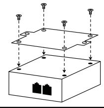
Line up the mounting plates and screw it on to the unit.
